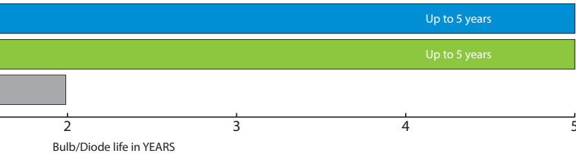
LEDs last 3 times longer than fluorescents — 5 years compared to 1.5 to 2 for T8s.
