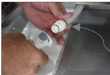
the quick connects on the hoses. Don't worry – it is normal for a few drops of the secondary fluid to escape when disconnecting the pans. It is a food grade solution that will not harm you or the case.
