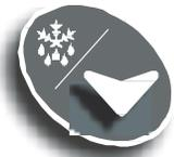
Push the **DOWN** key for more than 2 seconds and a manual defrost will start on the Dixell Controller. The controller must be turned back on when finished cleaning.
