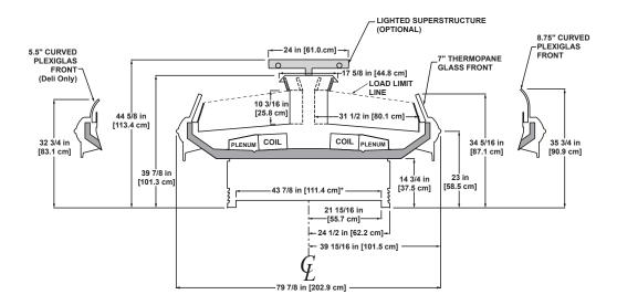
Please consult Hillphoenix Engineering Reference Manual for dimensions, plan views and technical specifications. Specifications subject to change without notice. Designed for optimal performance in store environments where temperature and humidity do not exceed 75°F and 55% R.H. Certified to UL 471 and ANSI/NSF Standard 7.
