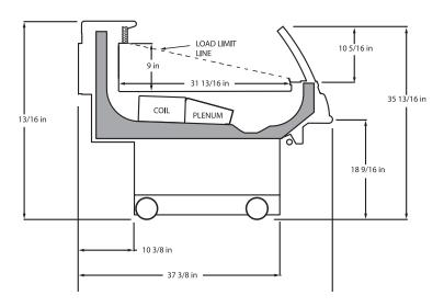
Please consult Hillphoenix Engineering Reference Manual for dimensions, plan views and technical specifications. Specifications subject to change without notice. Designed for optimal performance in store environments where temperature and humidity do not exceed 75°F and 55% R.H. Certified to UL 471 and ANSI/NSF Standard 7.
