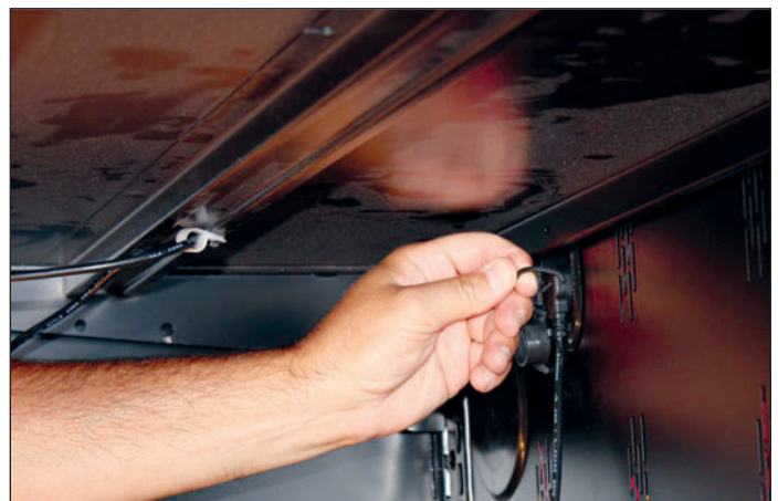
Fig. 10 Unplug the LED luminaire
