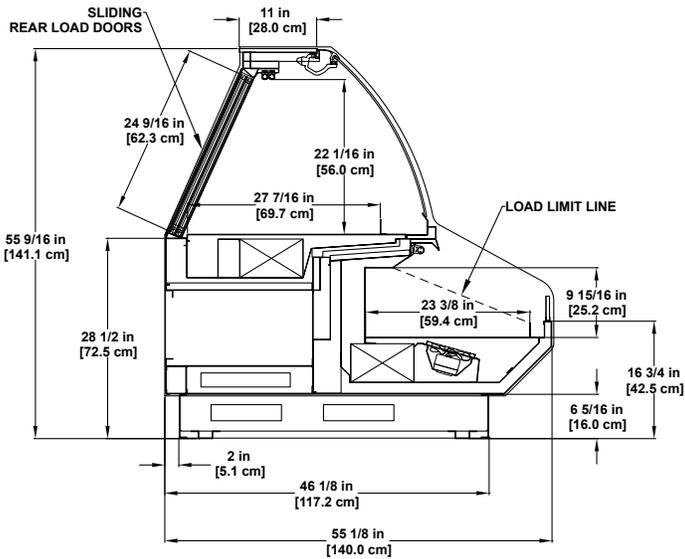
Please consult Hillphoenix Engineering Reference Manual for dimensions, plan views and technical specifications. Specifications subject to change without notice. Designed for optimal performance in store environments where temperature and humidity do not exceed 75 degrees and 55% R.H. Certified to UL 471 and ANSI/NSF Standard 7.
