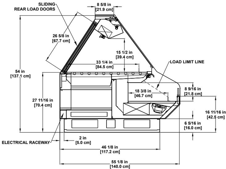
Please consult Hillphoenix Engineering Reference Manual for dimensions, plan views and technical specifications. Specifications subject to change without notice. Designed for optimal performance in store environments where temperature and humidity do not exceed 75 degrees and 55% R.H. Certified to UL 471 and ANSI/NSF Standard 7.
