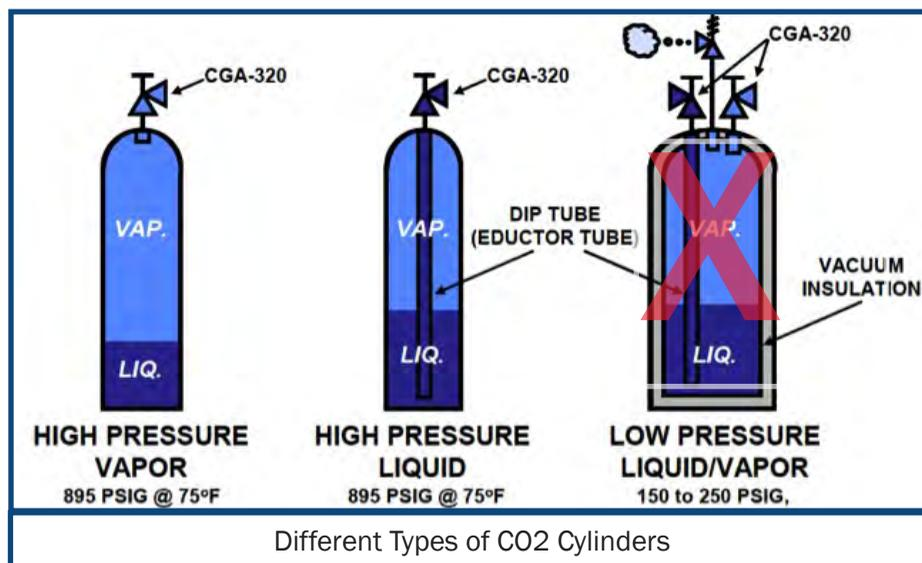
Note: Low-Pressure Liquid/Vapor cylinders are not recommended for use with booster systems due to their lower pressure ratings.
