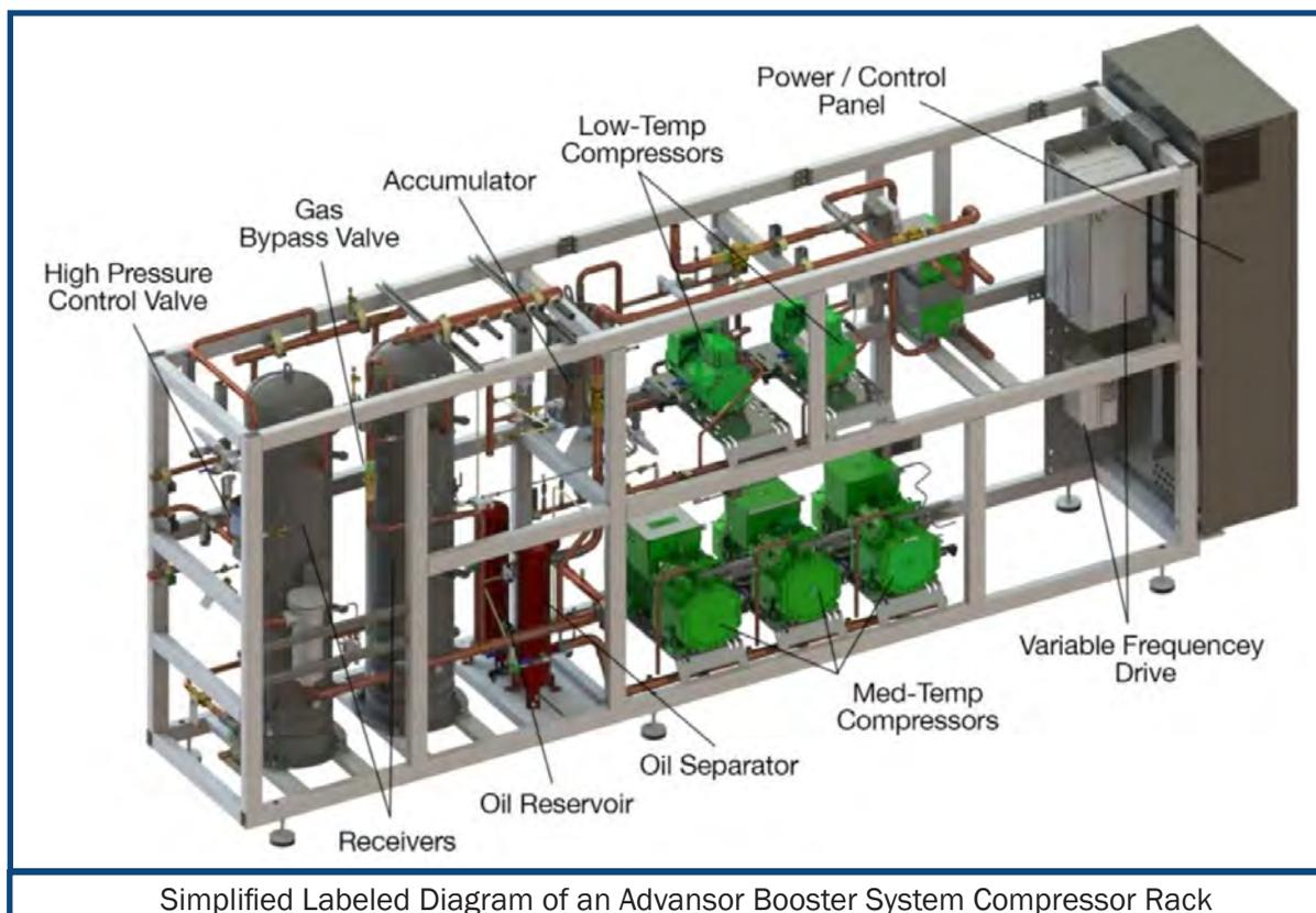
Advansor CO2 systems use many components that are common to other types of DX systems as well as some that are specifically designed for the application. Like any other DX type of system, the Advansor system relies on the four principle components which include compressors, evaporators, condensers and expansion valves.
