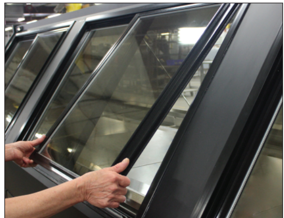
Fig. 16 Rear load door removal
