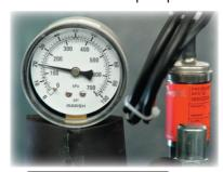
g. From this point on, maintain return fluid pressure at 20 psig by adding water as needed
