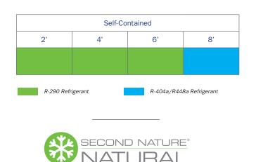
Second Nature® NATURAL environmentally friendly R-290 hydrocarbon refrigerant has an ozone depletion potential (ODP) of zero (0) and a global warming potential of three (3).
