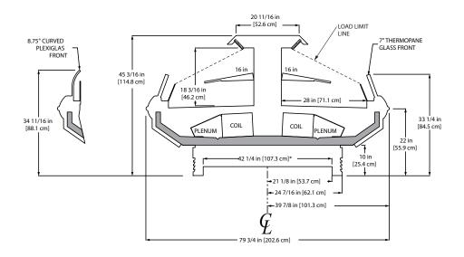
Please consult Hillphoenix Engineering Reference Manual for dimensions, plan views and technical specifications. Specifications subject to change without notice. Designed for optimal performance in store environments where temperature and humidity do not exceed 75°F and 55% R.H. Certified to UL 471 and ANSI/NSF Standard 7.
