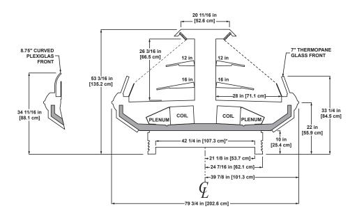
Please consult Hillphoenix Engineering Reference Manual for dimensions, plan views and technical specifications. Specifications subject to change without notice. Designed for optimal performance in store environments where temperature and humidity do not exceed 75°F and 55% R.H. Certified to UL 471 and ANSI/NSF Standard 7.
