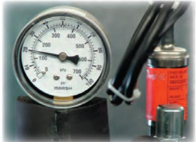
g. From this point on, maintain return fluid pressure at 20 psig by adding water as needed
