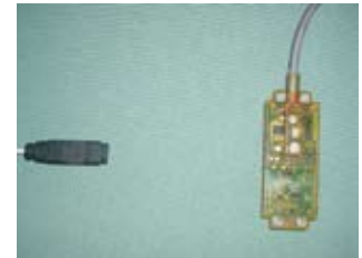
IR communication between USB port and control module
