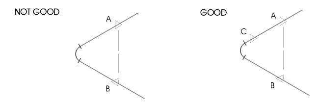
2. CORNERS MUST BE SUPPORTED and cannot be left free to pivot around the A-B axis as shown above.
