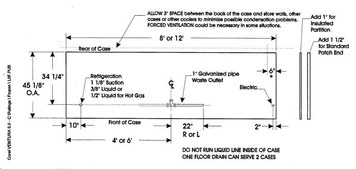
\* 208 Volt circuit is required at the top of this case for the defrost contactor
