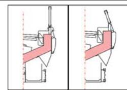
5-1/2" straight or 3-1/2" angled tempered thermopane glass front provide flexibility of front styling without reducing product visibility.
