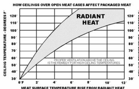
the cases. A dial thermometer stuck into the center of a piece of meat compared with one in the air stream quickly confirms this fact. Another fact is that the surface temperature of the meat will be higher than the center temperature due to radiant heat. TYLER's ongoing research identifies sources of radiant heat and accurately measures and records it. These charts were developed from the information gathered during this research. Two major sources of radiant heat are from
