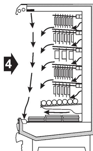
Figure 4 shows the proper air flow for cases with peg bars. The addition of a baffle above each row of peg bars, except the top row and a bottom shelf, maintains proper air flows and temperatures in the case. Non-load bearing air baffles should run the same width as the peg bars.
