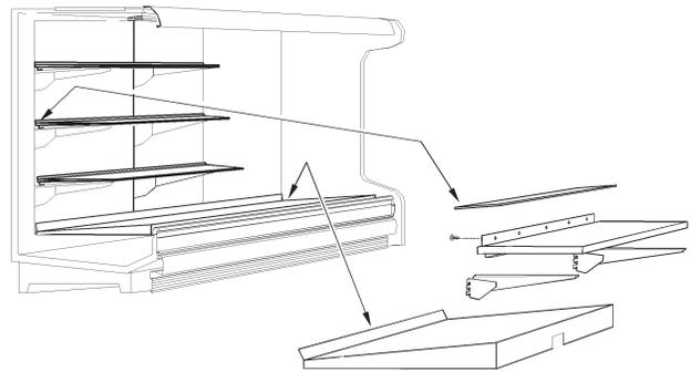
All egg shelves come galvanized or stainless steel. The upper egg shelves are 15" x 48" and come with 82 degree fixed white brackets. The brackets are available in one position only. The upper egg shelves assemblies include a rear air close-off.
