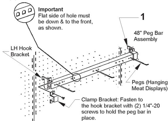
1. 48" peg bar with 52 holes to accept pegs. Flat side of holes in peg bar must be down and to the front of the bar. Attach two hook brackets to peg bar with two clamp brackets and four screws. Position and install peg bar in slotted holes in back of case.
