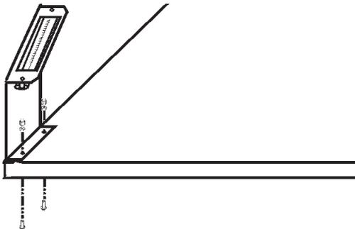
4. Mount the bracket to the bottom tray with two screws, washers and capnuts.
