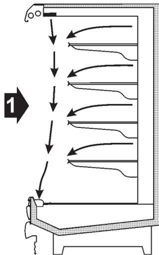
Figure 2 shows what happens to the air flow when the shelves are removed. The air drifts back to the rear duct and swirls about. This breaks the protective barrier, causing the case air to mix with ambient air to a great extent.
