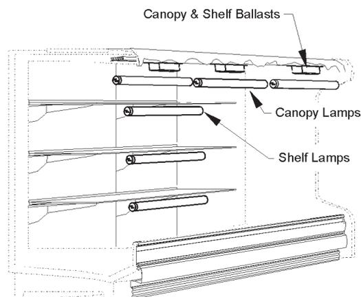
All light ballasts are located under the canopy and mounted above or on the top of the canopy light channel. This includes remote ballasts for optional shelf lights and optional nose lights. The canopy light(s) are under the canopy light channel in the top of the case. The optional shelf lights are mounted under the top interior liner above each shelf section.
