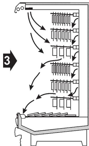
When the bars are fully stocked, the effect is minimized, but product temperatures will not be as good as they could be. Sweating may be noticed on the top duct panel above the bars. The coil will also frost faster, requiring more frequent defrosts.
