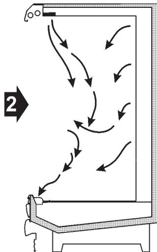
Figure 3 depicts what happens to the air flow in a case full of peg bars. The air falls through openings between packages and fails to maintain a protective barrier. When the bars are fully stocked, the effect is minimized, but product temperatures will not be as good as they could be. Sweating may be noticed on the top duct panel above the bars. The coil will also frost faster, requiring more frequent defrosts.
