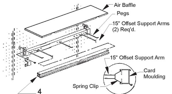
**Card Moulding:** Plastic or Brite Shiny Aluminum. Slides onto the two Offset Support Arms.
