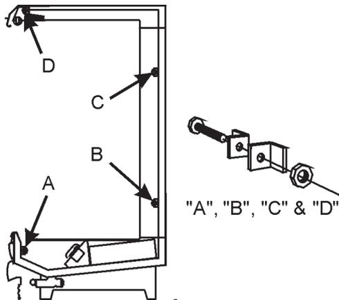
All N7DNHPL and NHDHP models have four pull-ups at each end of the case. Pull-ups A, B, C and D are located as shown and should be installed and tightened starting with A and finishing with D.
