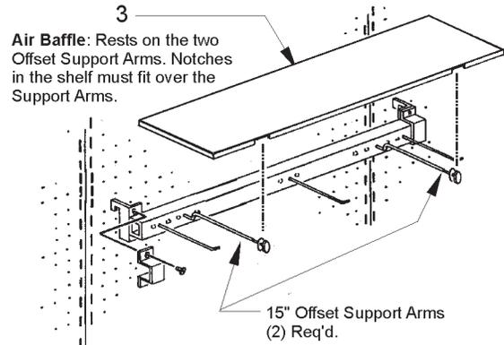
3. Non-load bearing air baffle should run the same width as the peg bar. Air baffle rests on the two offset support arms. The notches in the air baffle must fit over the support arms. **NOTE: The air baffle should be solid in design and positioned 1" in front of the rear duct and 5.5" back from the rear edge of the card moulding.**
