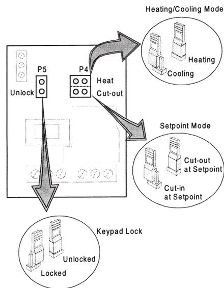
3. Set the Heating/Cooling jumper blocks to the "COOL" position.
