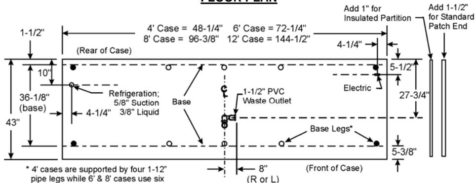
\* 4' cases are supported by four 1-1/2" pipe legs while 6' & 8' cases use six 1-1/2" pipe legs and 12' cases use eight 1-1/2" pipe legs.
