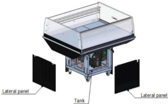
Fig. 15 Removing condensating unit panels
