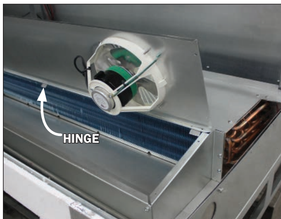
Fig. 20 Pressure plate and hinges (underside)
