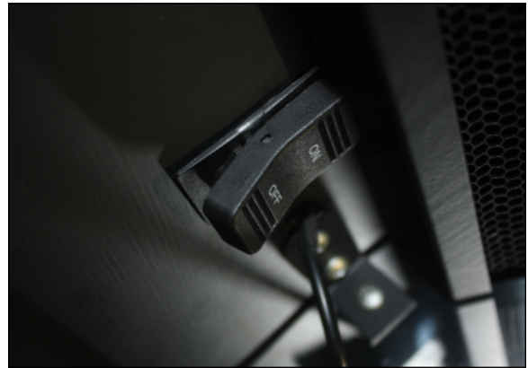
Fig. 12 Upper cornice light switch
