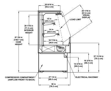
Please consult Hillphoenix Engineering Reference Manual for dimensions, plan views and technical specifications. Specifications subject to change without notice. Designed for optimal performance in store environments where temperature and humidity do not exceed 80° F and 55% R.H. Certified to UL 471 and ANSI/NSF Standard 7.
